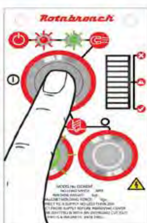
2) Magnet ON To turn the magnet ON or OFF, depress the large button on the control panel. A GREEN LED will indicate the magnet is ON.
