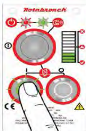
4) Motor ON Press the GREEN Switch to turn the motor on. Proceed with cutting - following all safety guidelines.
